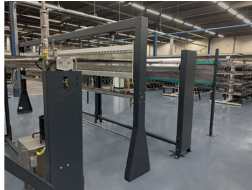
Leasing device with heddles and auxiliary equipment
