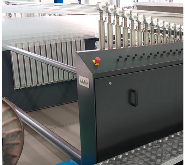
Newly designed leasing device (pneumatic)
